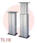
Max. load 4,500N (push) Self-locking force 4,500N Max. dynamic bending moment 250Nm Max. speed at max. load 6.6mm/s Max. speed at no load 45mm/s Retracted length ≥ Stroke + 147mm
